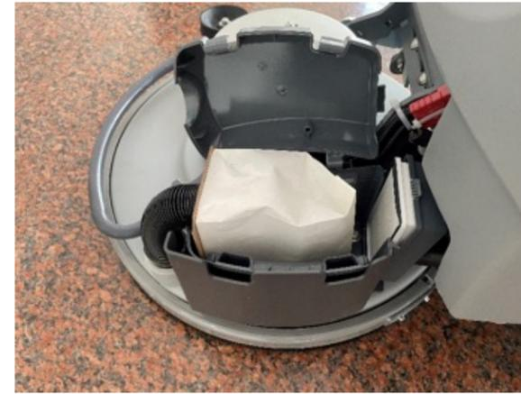
3. Install dust bag and filter as shown. Replace cover.
