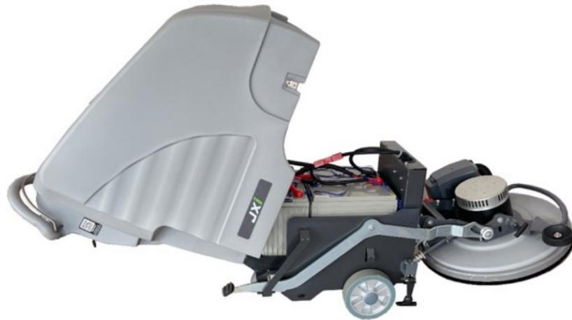
3. Connect the cables to the battery posts as shown. Connect the machine's black(-) battery cable last. Use insulated tools when working near batteries.
