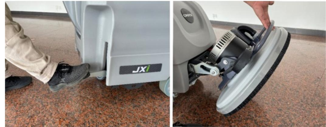
3. Install the burnishing pad on pad driver and Secure pad with center-lock. Do not operate machine without pad center-lock installed.
