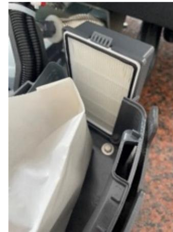
4. The filter required to be replaced every 200hrs of use.
