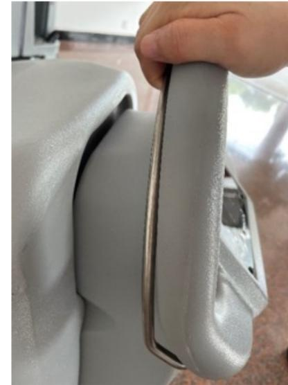
5. To stop burnishing, release the start bail. The machine stops burnishing when the bail is released.
